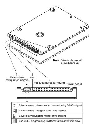
Figure 2. Connector and master/slave jumper setup
