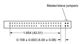
Figure 5. ATA Interface connector dimensions (non-SFF dimension, for reference only)
