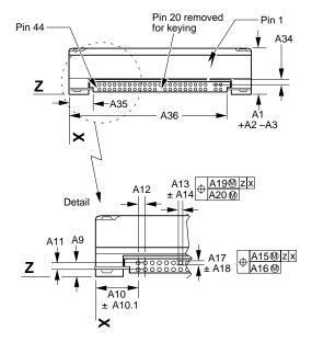
Figure 4. Drive mounting dimensions—end view (for dimension specifications, see table below).
