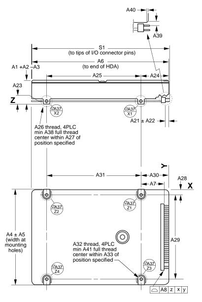
Figure 3. Drive mounting dimensions—side and bottom view (for dimension specifications, see table on pages 21 and 22).
